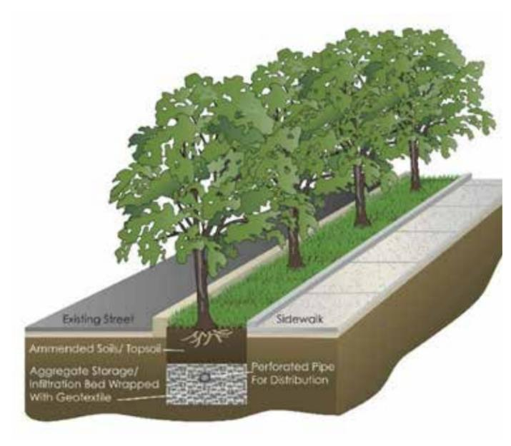
*Tree pits can help manage stormwater runoff from sidewalks and provide shade*
