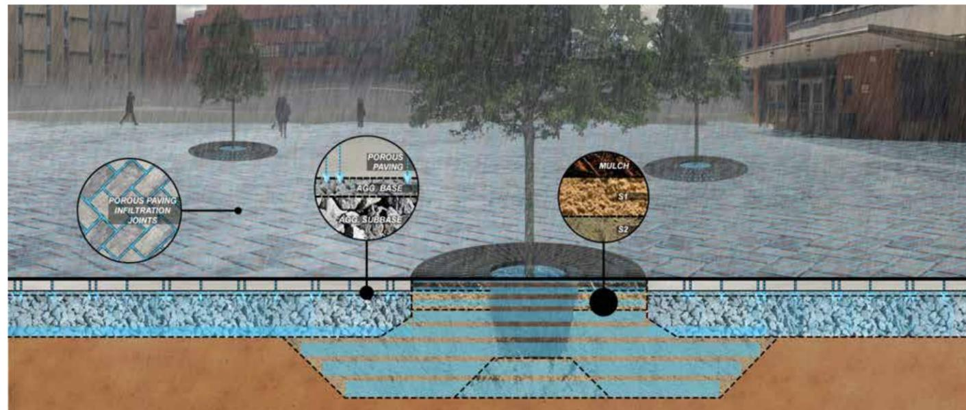
Planter boxes help delay and limit stormwater runoff
