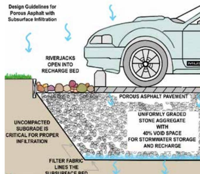
*Pervious asphalt allows for localized infiltration and limits stormwater runoff*
