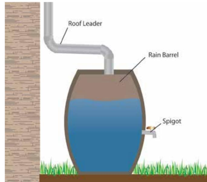
*Rain barrels and cisterns limit stormwater runoff and allow it to be stored for future use*
